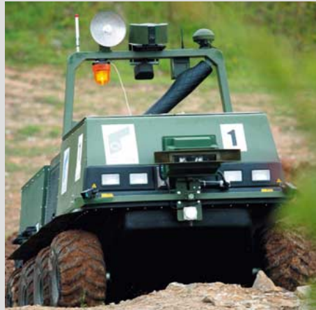
Substitution systems from Rheinmetall Defence for high-risk missions: Trobot with the integrated Smover concept and the radio-controlled Foxbot from RDE, Bremen.
