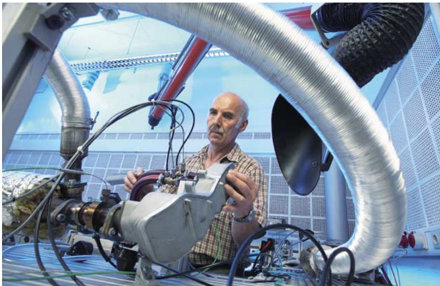
Test routine at the cooler test stand : test stand mechanic Günter Thiel shown here making the preparations for performance measurements on the die-cast aluminum EGR cooler. The sophisticated design of this unit allows the introduction of up to 800°C hot exhaust gas which is then cooled down to around 180°C.
