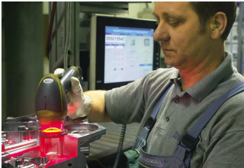
Clearly identified: with handheld camera, ATAG employee Albert Grötzinger captures the data matrix code embossed on to the engine block. The crankcase identification number is then relayed to the PDA terminal shown in the background.
