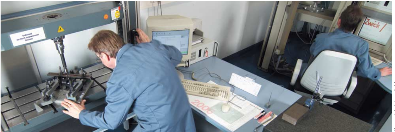
A routine day for measurements at Pierburg: technician Peter Schlabs (left) and coworker Rolf Schnakenberg measuring the pull-off forces of bearing retainers for a convertible hood frame. Here the adhesive bond between bearing support and retainer is being tested.
