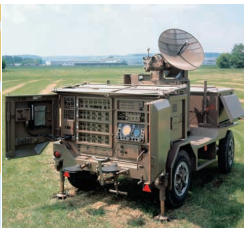
Tracking migrants: in the comprehensive project launched by the Swiss ornithological station Sempach, the Superfledermaus radar system of Zurich-based Oerlikon Contraves (OC) will be used to trace the movement of birds across the desert and along the coast of Mauritania. The system is being equipped with new logarithmic amplifiers and PC-based registration systems.
