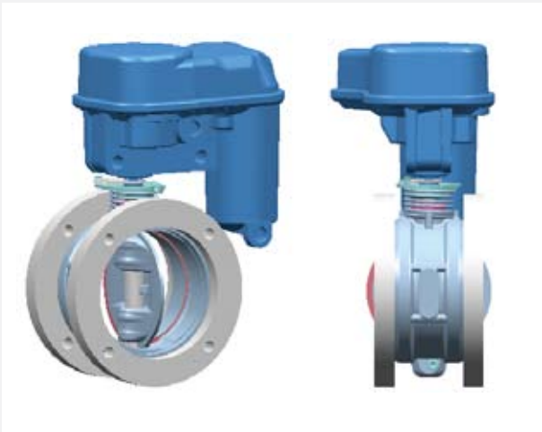
Fig. 6 and 7: Example of an electrically actuated exhaust flap for use in two-stage sequential turbo-charging
